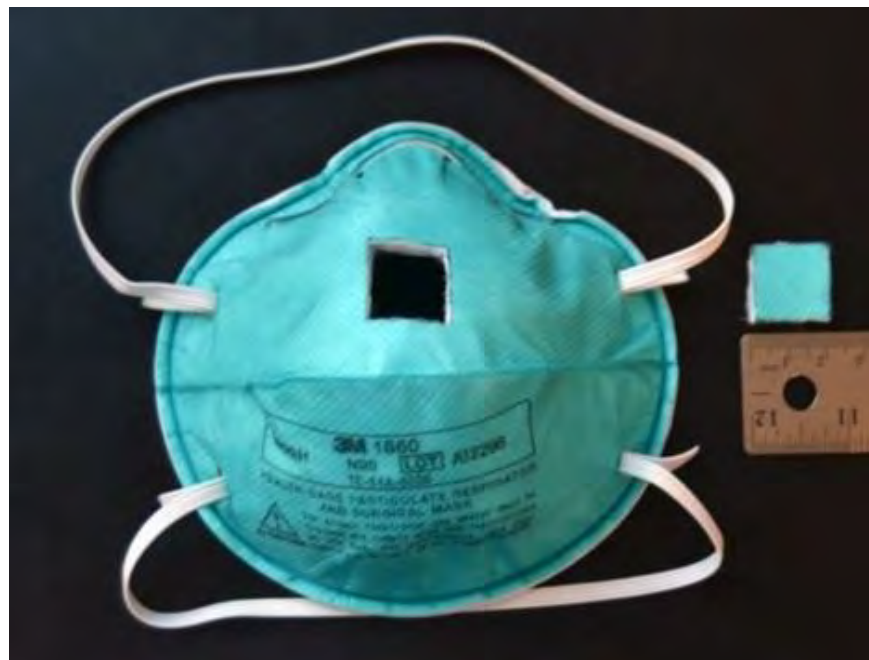
Figure 5. 3M 1860 N95 FFR with 2 cm x 2 cm Swatch Excised
