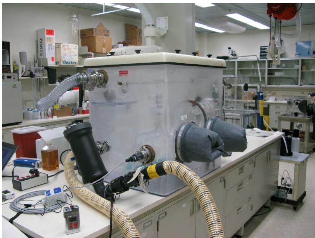
Figure 6. HPV Exposure Chamber
