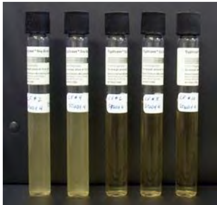
Figure 7. Representative Fractionation Test Results Comparing Turbid (Growth) and Clear (No-Growth) Samples
