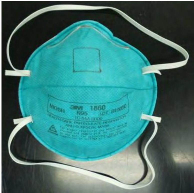
Figure 8. N95 FFR with Marked Area for Contamination
