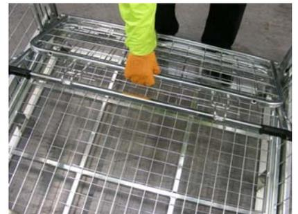
Lift the top folding section up and hinge down to sit flat against the FSC base. Step in if required.
