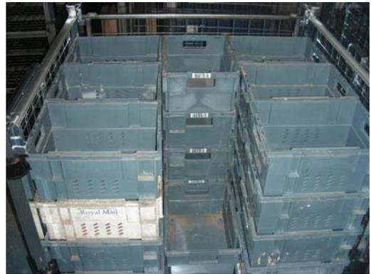
When loading or unloading stackable items, strapped bundles, cartons or loaded trays it is recommended that the full depth hinged gates are opened and secured to cage sides using the bungees provided. Load against the closed hinged gates.
