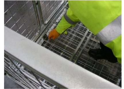
Firmly grasp the LH side panel and carefully lift it until the lower support legs are clear of the base and fold forward, lowering it over the folded gate.
