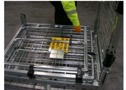
Firmly grasp the RH side panel and carefully lift it until the lower support legs are clear of the base and fold forward, lowering it over the folded LH side.
