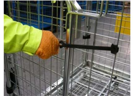
Hinge open LH full gate, secure against side panel with bungee strap.
