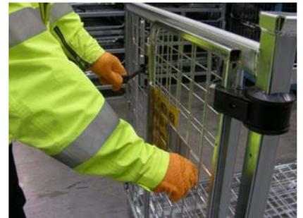
Lift out the top folding section of the folding gate, hinge outwards and fold down over lower half of gate.
