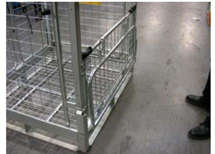
Using both hands slide the lower gate release catches inwards to release them from the outer posts. Lower the folded gate assembly into the FSC.
