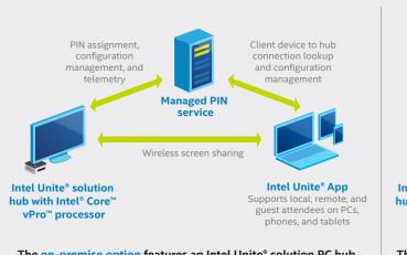
The on-premise option features an Intel Unite® solution PC hub, managed PIN service, and the Intel Unite client app
