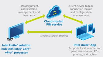
The Intel Unite® Cloud Service option connects directly to the Intel Unite solution hub PC and supports the Intel Unite client app
